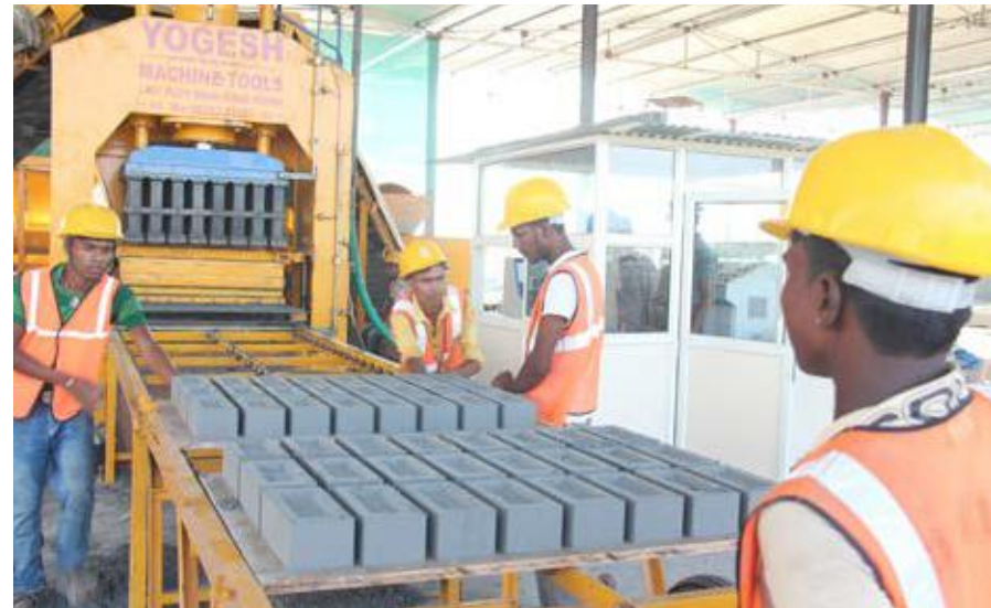
Locally sourced fly ash was used to manufacture the FALG (fly ash) bricks on site
